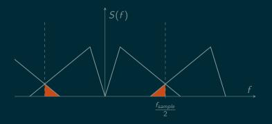
For real-valued sampling, the observed bandwidth of the analog signal must be limited to less than half the sampling rate.
