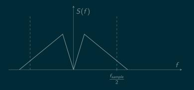
For real-valued sampling, the observed bandwidth of the analog signal must be limited to less than half the sampling rate.
